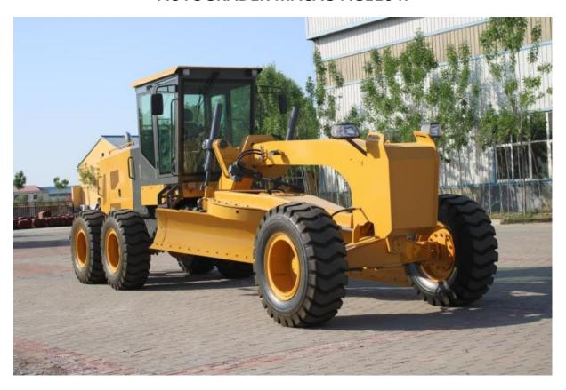
Min. ground clearance of front axle: 560 mm
